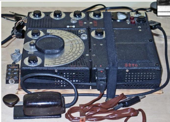
A 12WG with accessories as kept in the DHM (Left). Note the use of a WW2 'mouse' Morse key and accumulator charging resistor left in front of the receiver.
